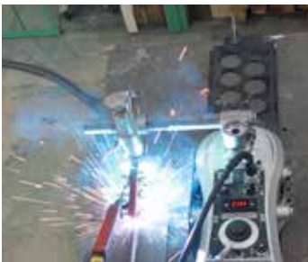
IK-12 NEXT straight welding
