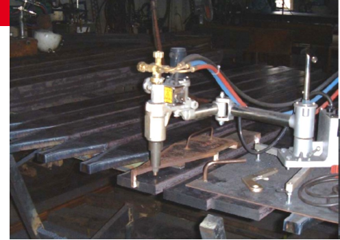
IK-82 M300 being used for profile cutting
