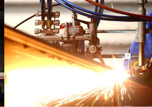
Chamfering (1:4 ratio bevelling) using single torch
