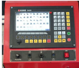
D420 controller includes a 48 shape library and a simple to use interface.
