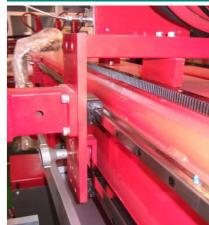
High-speed accuracy is achieved with linear guide ways and slides to the X-direction main drive carriage and sub-carriages.
