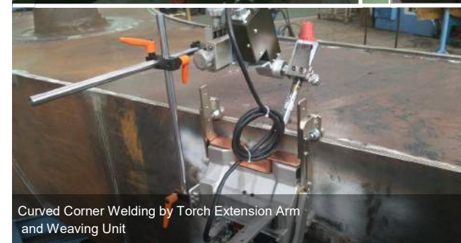
Corner Welding by Edge Imitation Guide Roller and Torch Extension
