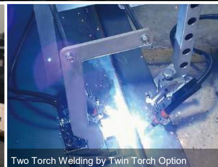
Two Torch Welding by Twin Torch Option
