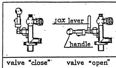
(Now, the preheat oxygen gas and fuel gas can flow.)
