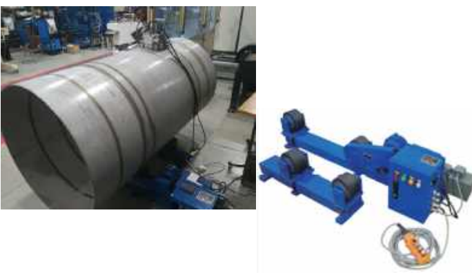
Combination of welding carriage and turning roller
