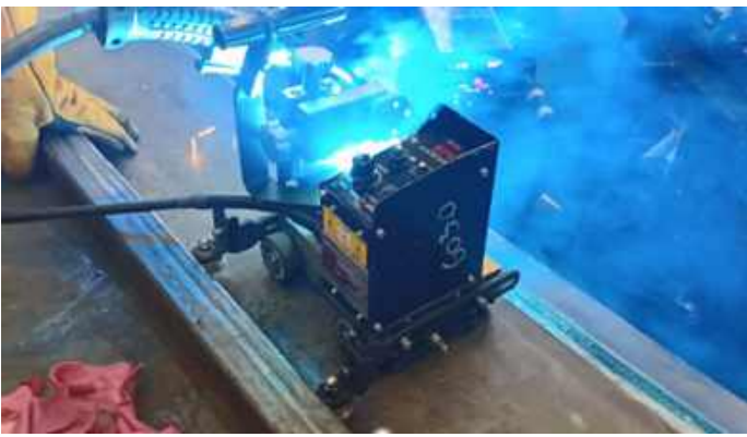
Flipping guide rollers to trace at back side
