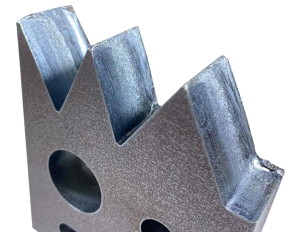
12kW Fiber Laser Cutting Material: SN490C 25mm
