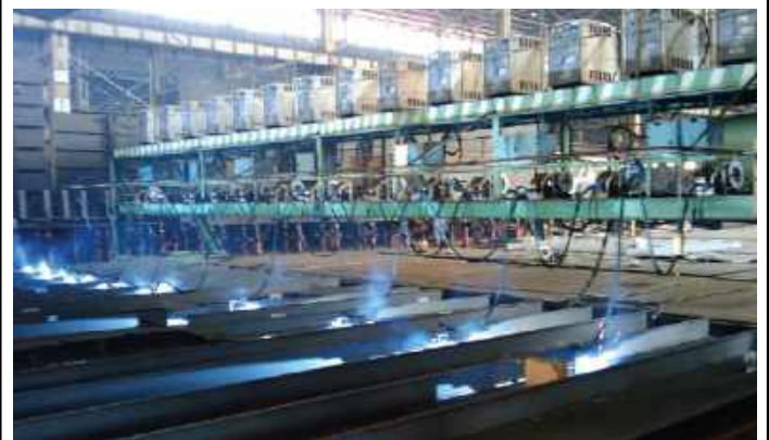
Fillet welding gantry system
